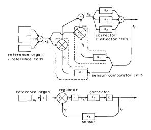
Fig. 6. Multicellular feedback system with lumped sensor-comparator cells (above) and its representation by additional serial gain elements (below)
